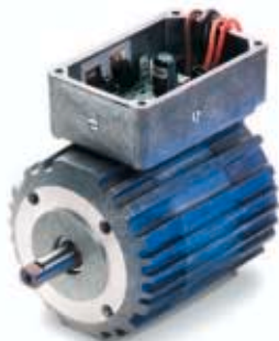
Type "34B/FV" BLDC motors and gearmotors with built-in custom speed controls. Easy operation and connections, PWM speed signal, 24-36 VDC, 5 VDC logic signal, and tach pulse output.
