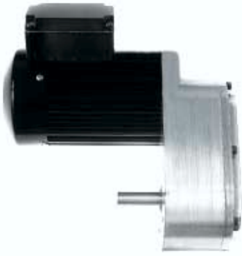
Low-profile "HG" gearmotor for high torque in tight spaces (up to 1000 lb-in). Applications: conveyors, ice machines, and machine tools. Gearhead available with AC, DC, or BLDC motors.
