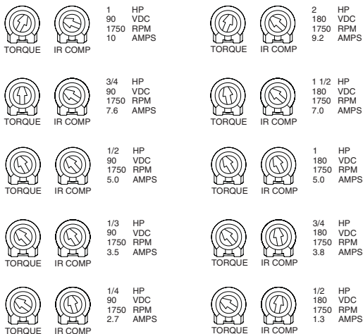
Figure 19. Recommended TORQUE and IR COMP Settings
