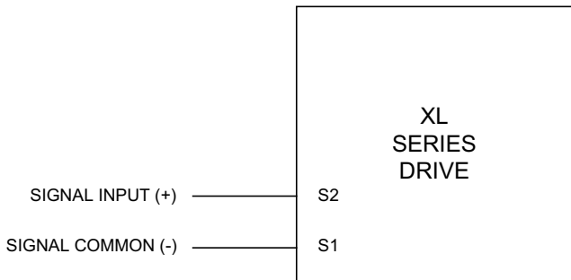
Figure 6. Voltage Follower Connections
