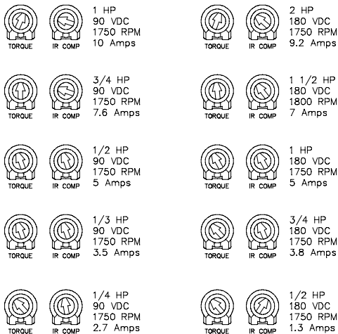
Figure 16. Recommended Torque and IR COMP Settings (actual settings may vary with each application)
