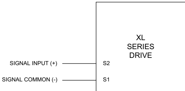
Figure 6. Voltage Follower Connections
