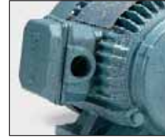
Conduit Box Rotation Note: Conduit box remains in same location and is rotated in 90° increments.
