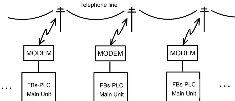
Besides the above area network connection, FBS-PLC can also be connected using MODEM via the phone line (either leased line or public phone line) to form remote multiple PLC Link. (When using a public phone line, the Master PLC will perform consecutive dialing for all its Slave PLC.)
