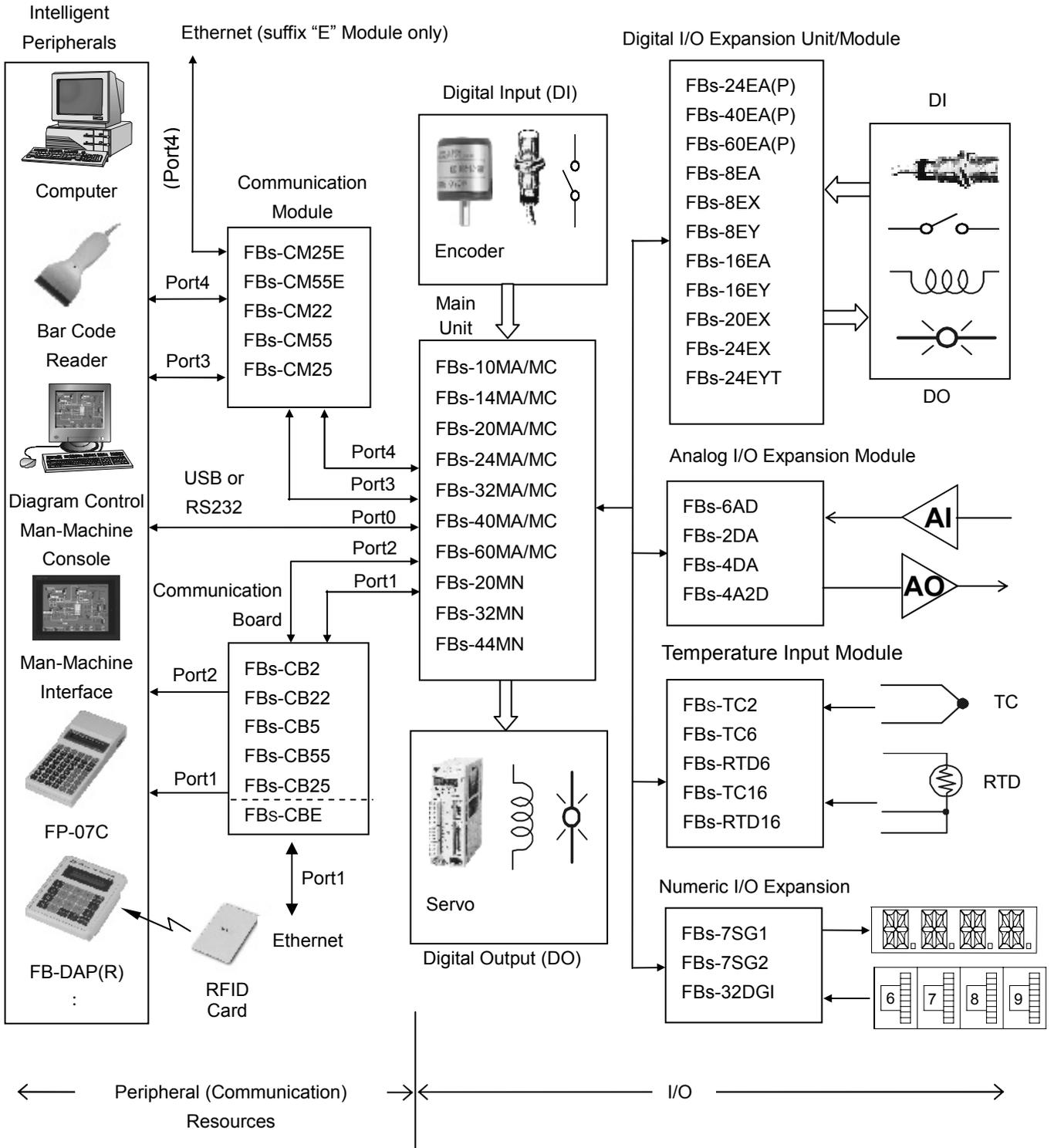
For the I/O of FBs-PLC, it can achieve a maximum of 256 point digital input (DI), 256 point digital output (DO), 64 word numeric input (NI), and 64 word numeric output (NO). Combined with various special interface modules, it can directly connect with devices such as Thermocouple, RTD, 7-segment LED display, and the Thumbwheel switch, which are shown on the right in the above figure.
