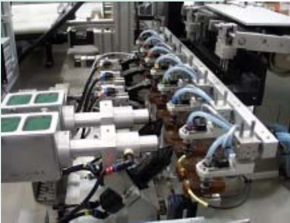
Ismeca's new capacitor testing machine — note the eight pick-and-place stations.
