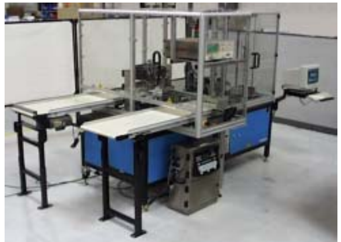
Ismeca's new capacitor testing machine — note entry and exit conveyors at left, LCR test instruments at top, and HMI at right.
