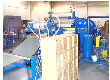
Feed bins for molding compound raw materials at process start
