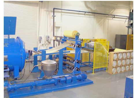
Plastic carrier sheet unwinds to bring raw materials into molding compound process
