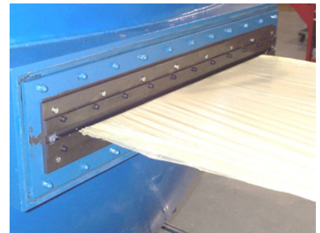
Molding compound sheet exits process and on to take-up reel
