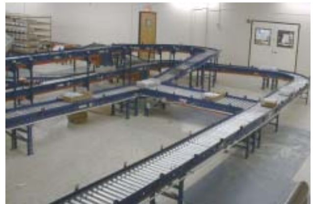
Conveyors sort mail via cross-over path for a second pass through the machinery.
