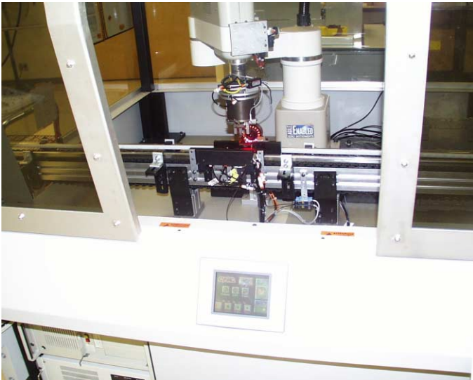
At Station 1: Robot places heat sink on carrier for subsequent assembly
