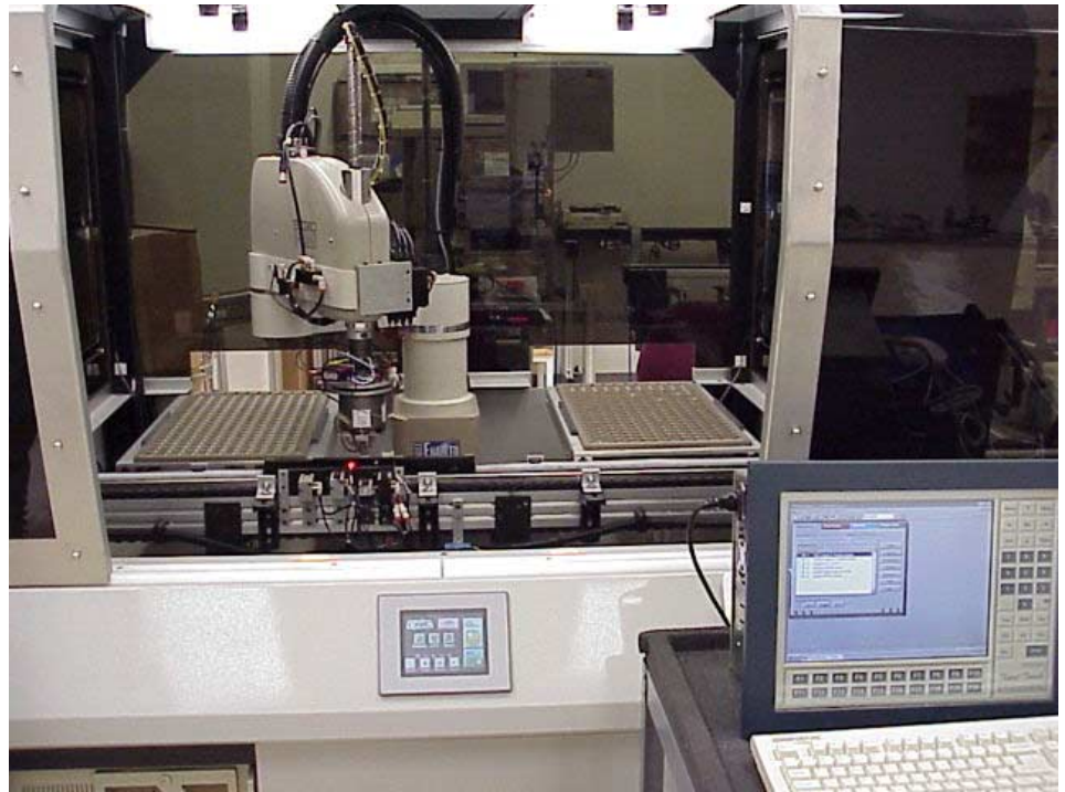
C-MAC's electronic control module line during project development, with industrial PC (lower right) displaying Think & Do's ProjectBinder
