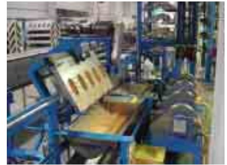
After hot gell soak, the machine pours out excess latex.
