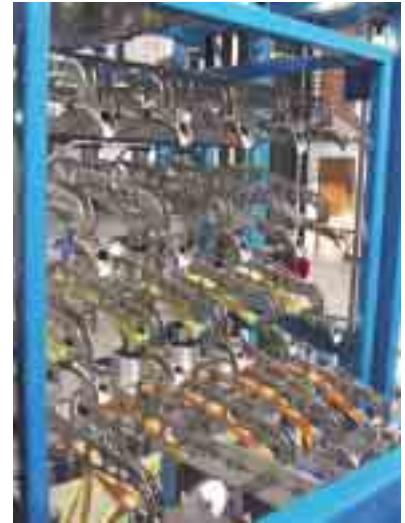
Latex filling station fills five molds with one of four colors.
